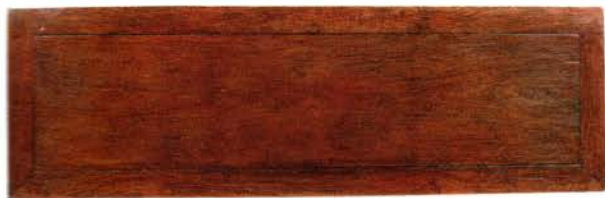
案面以格角榫造法攒边框，打槽平镶木纹华美的独板面心 The top is of mitre, mortise and tenon frame construction with a well grained single board tongue-and-grooved, flush floating panel
