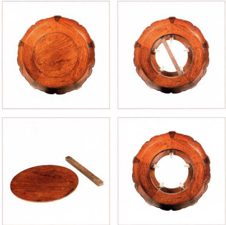
几面圆边框用楔钉榫五接，装独板活动心板，下安一根可装可卸的托带嵌入边框支承 The top frame of five sections, held together by pressure-pegged scarf joints with a single board centre panel, supported by an underneath brace resting on ledges in the frame members Both centre panel and support brace are removable
